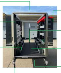
Side extensions for optimum adaptation to the vehicle width
